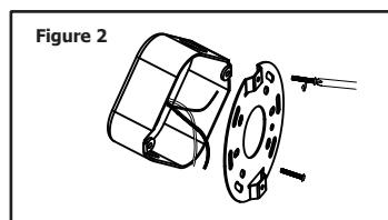
2. Attach the Base Plate to the junction box with the screws.
