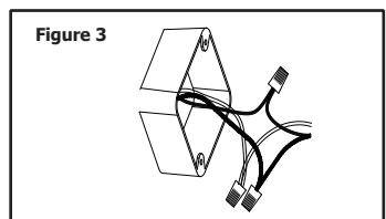
3. Connect the LED fixture to 120-277 VAC 60Hz in accordance to local codes, support fixture while making connections.
