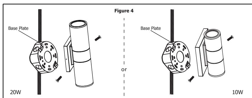
4. Align mounting holes of lamp body to base plate and secure with provided fasteners.
